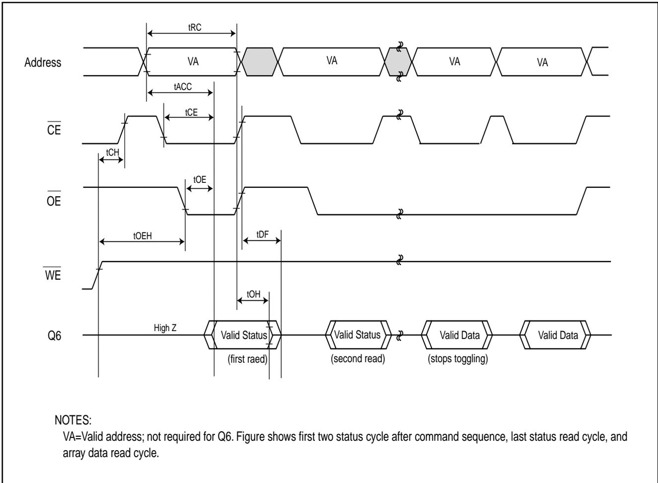
Fig 16. TOGGLE BIT ALGORITHM
