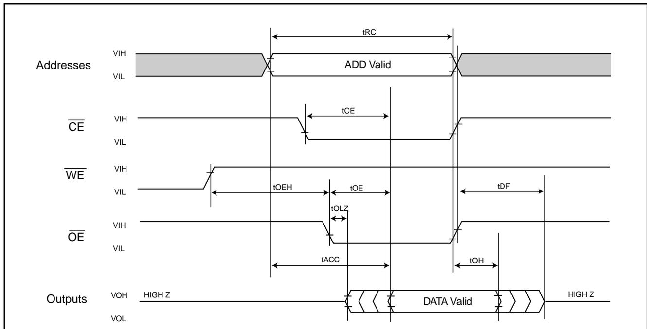
**AC CHARACTERISTICS TA=0°C to 70°C, VCC=3.0V~3.6V**
